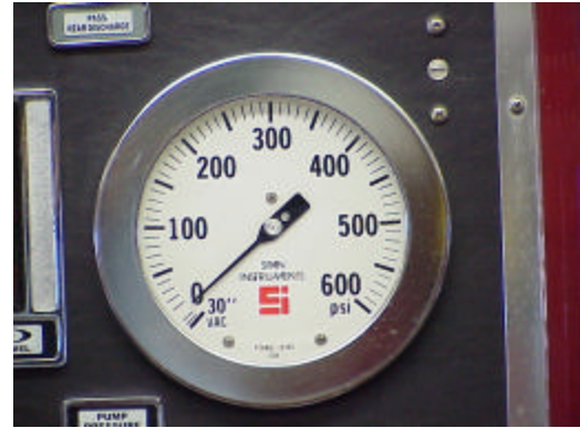
Figure 14: Main pressure gage. Note the gage face that shows inches of Mercury.
