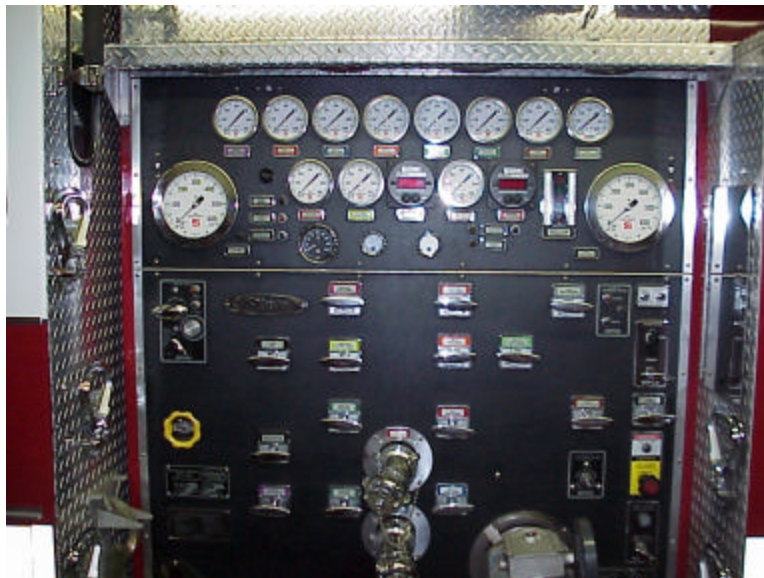
Figure 12: Picture of the Compound gage and the main pressure gage.
