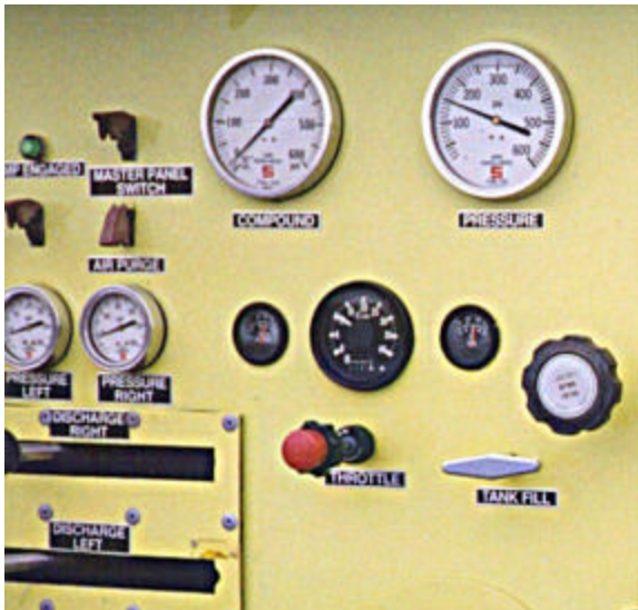
Figure 15: Pump panel with only one Compound gage. Only gage with Inches of mercury on gage face.
